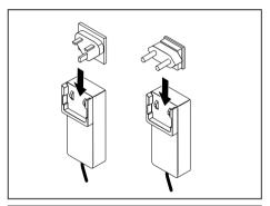
► Take the plug which is approved for the country in which the device will be used and insert it into the mains adapter.
